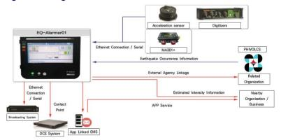
Earthquake alarm device with a P-wave early warning algorithm
