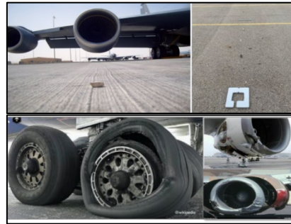
Damage caused by FODs
